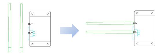
3° Plug the interlock cable and connect it to a power supply (100-240 VAC). This device has no buttons or switches so, once it is powered, it should start running.
